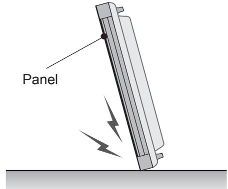
If the product is tilted onto the bezel, the bottom of the panel may be damaged.
