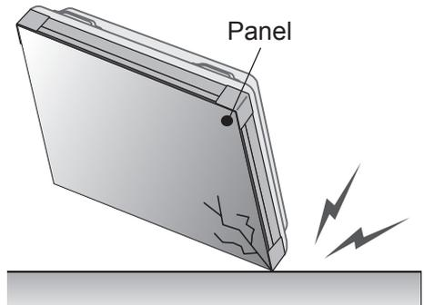
If the product is tilted onto the edge of the panel, the panel may be damaged.
