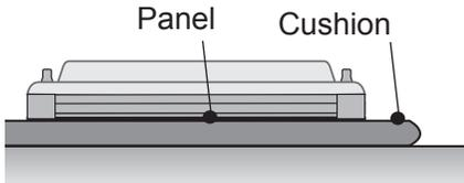
When laying down the product, lay a cushion on a flat floor. Put the product on it with the panel of the product facing down.
